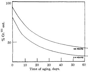
Fig. 3.—Diffusibility of 8.40  $\times$  10<sup>-3</sup> M chromic acetate in  $\mu = 0.1$ , phosphate buffer at 5–8° (pH 7.35).
