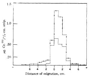
Fig. 1.—Paper electrophoresis of chromic acetate in  $\mu = 0.1$ , phosphate buffer pH 7.35: I (—), 4.36 × 10<sup>-3</sup> M; II ( $\rightarrow \rightarrow$ ), 6.44 × 10<sup>-3</sup> M.
