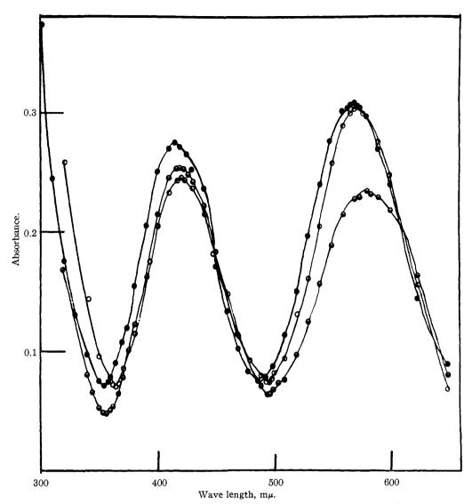
Fig. 5.—Absorption spectra of 8.19  $\times$  10<sup>-8</sup> M chromic acetate at various pH's: (I) O, pH 4.86; (II)  $\bullet$ , pH 6.30; (III)  $\hat{\bullet}$ , pH 11.20.
